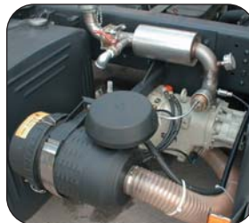
Cmax2 R 35 with Transmission prop shaft driven
