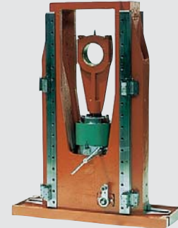
16 roller rotary elements hydraulic overload safety device with combined ram adjustment
