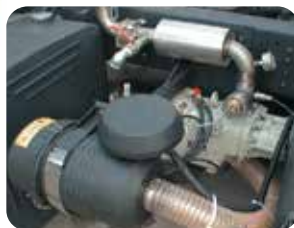
Cmax 2 R 35 with transmission prop shaft driven
