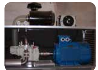
Cmax 2 R 35 sound proofed stationary unit electrically driven
